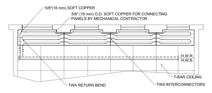
TWA RADIANT PANELS NOTCHED AROUND PERIMETER COLUMNS, EVEN PASS COILING SHOWN
