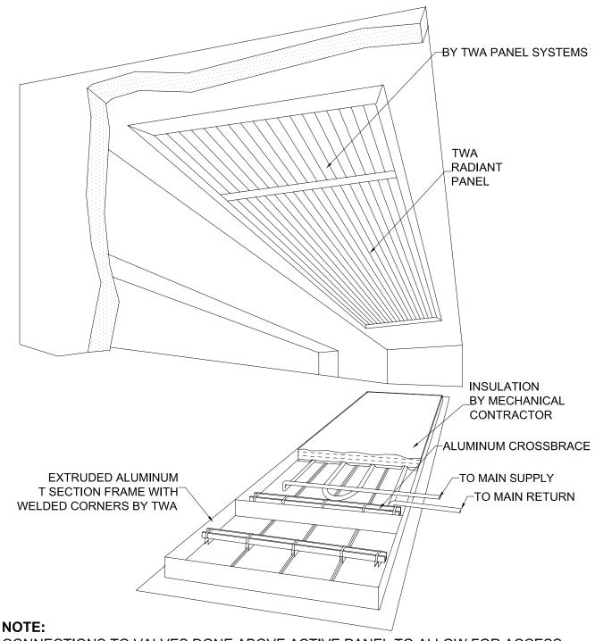
CONNECTIONS TO VALVES DONE ABOVE ACTIVE PANEL TO ALLOW FOR ACCESS PANEL PLACEMENT. OPENING FOR RADIANT PANEL OBTAINED FROM L-7.
