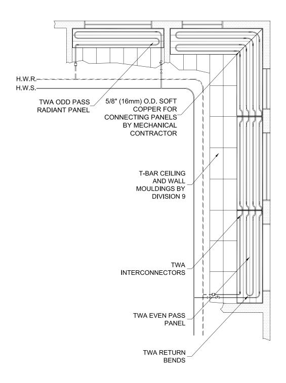
PIPING DETAIL FOR ODD AND EVEN PASS LINEAR PANELS
