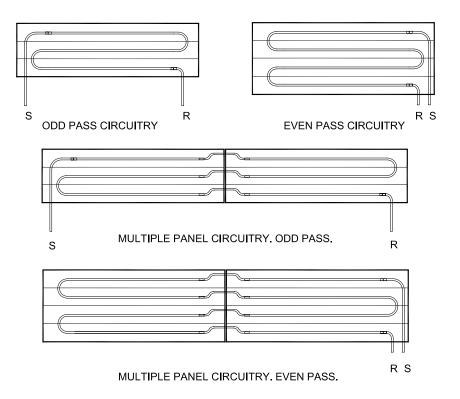
Single panel length to a maximum of 16 feet (4877 mm). Pressure drop for Twa Panel Systems, Inc. 5/8" (16 mm) O.D. tubing:
