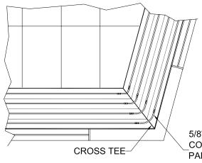
5/8" (16 mm) O.D. SOFT COPPER FOR CONNECTING PANELS BY MECHANICAL CONTRACTOR
