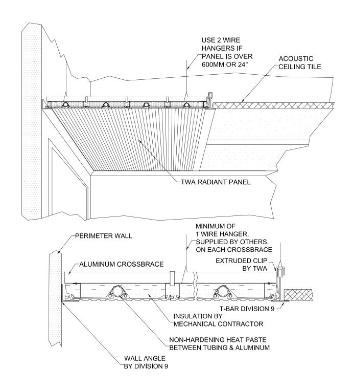
NOTE: OPENING FOR RADIANT PANEL OBTAINED FROM L-7.
