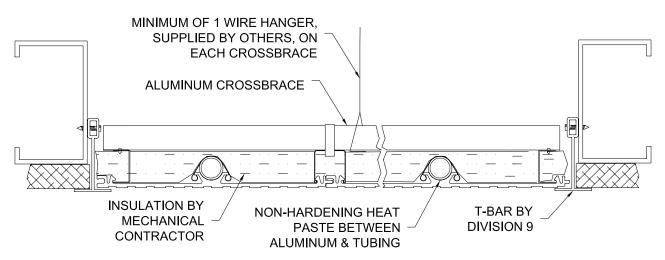
**NOTE:** OPENING FOR RADIANT PANEL OBTAINED FROM L-7. ACCESS TO SUPPLY, RETURN AND INTERCONNECTION
